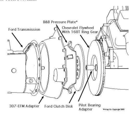
ASIDE FROM WHAT IS INCLUDED IN YOUR WILCAP ADAPTER KIT, THE ADAPTER IS DESIGNED TO USE THE 49-53 10" MERCURY PRESSURE PLATE (P/N 305993) WITH THE B&B PATTERN AND THE 10" CLUTCH FORD DISK. THE STOCK THROW OUT BEARING FROM YOUR TRASMISSION IS USED. THE ENGINES STOCK FLYWHEEL (168 TOOTH RING GEAR WITH 10.5"
